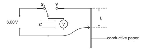
The switch is moved from X to Y, and the time t for the potential difference across the capacitor to halve is measured.
