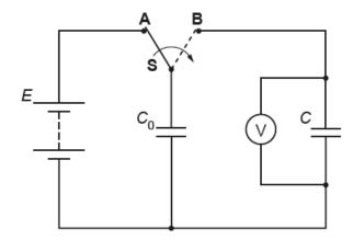
The switch  ${\bf S}$  is then moved to position  ${\bf B}$ . The initial charge stored by the capacitor of capacitance  $C_0$  is shared between the two capacitors. The final reading on the voltmeter is V.
