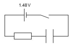
The electromotive force (e.m.f.) E of the cell is 1.48 V and it has negligible internal resistance. The resistance of the resistor is  $120\,\mathrm{k}\Omega$  and the capacitance of the capacitor is  $2000\,\mu\text{F}$ . At time t=0 the capacitor is uncharged.
