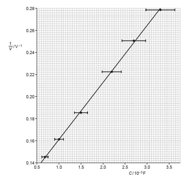
The gradient of the line of best fit is  $51 \text{ V}^{-1} \text{ F}^{-1}$ . The value of *E* is 9.1 V.
