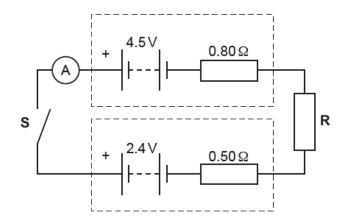
The positive terminals of the batteries are connected together.
