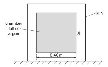
The internal chamber is a cube. Each side of this cube has length 0.46 m. The chamber is sealed and full of argon. Argon behaves as an ideal gas.
