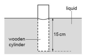
The length of the cylinder below the liquid level is 15 cm.
