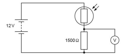
The fixed resistor has resistance  $1500 \Omega$ .
