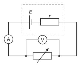
The student changes the resistance of the variable resistor. The potential difference *V* across the variable resistor and the current *I* in the circuit are measured.
