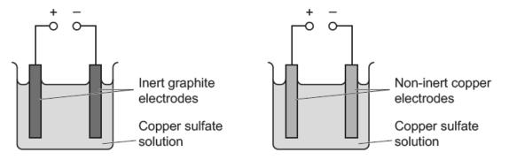
(a) In both experiments, copper is deposited at the cathode.
