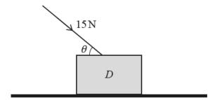
A block D of weight 50 N lies at rest in equilibrium on a fixed rough horizontal surface. A force of magnitude 15 N is applied to D at an angle  $\theta$  to the horizontal (see diagram).
