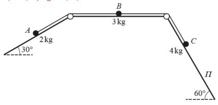
One end of a light inextensible string is attached to a particle A of mass 2 kg. The other end of the string is attached to a second particle B of mass 3 kg. Particle A is in contact with a smooth plane inclined at 30° to the horizontal and particle B is in contact with a rough horizontal plane.
