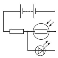
The LED is very close to, and facing the light dependent resistor (LDR). The circuit is taken into a dark room.
